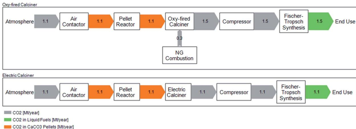
Fig. 2 Flows of carbon (reported as equivalent masses of  $\text{CO}_2$  for liquid fuels and  $\text{CaCO}_3$  pellets) for the oxy-fired (top) and electric (bottom) calciner in the direct air capture and Fischer–Tropsch process.
